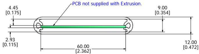
Extrusion designed for 60mm wide x 80mm long PCBs.
