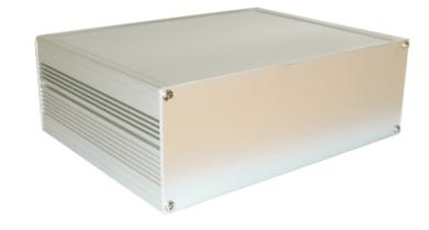
The profile housing PG 1 consist of two strong side profile, top- and bottom plate and two end plates (2,5mm). The construction of the side profile includes different slots for mounting power devices like amplifiers or power transistors and for plug in PCB and plates.
