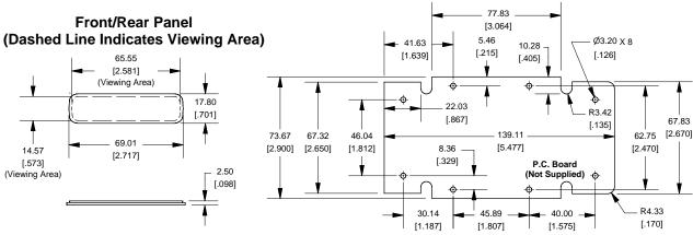
Enclosures can be Factory Modified (Milling, Drilling, Printing etc.) Solid models of this enclosure available in STEP or IGES.
