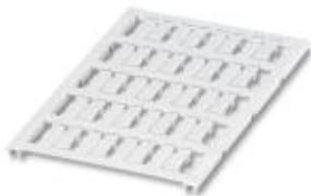
Conductor marker, Sheet, white, Unlabeled, Can be labeled with: BLUEMARK CLED, BLUEMARK LED, Plotter, Mounting type: Clip on, Cable diameter: 1.2-1.9 mm, Lettering field: 15 x 4 mm
