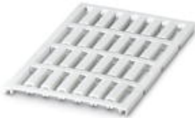
Conductor marker, Sheet, white, Unlabeled, Can be labeled with: BLUEMARK CLED, BLUEMARK LED, Plotter, Mounting type: Slide on, Cable diameter: 3.6-4.9 mm, Lettering field: 21 x 5 mm
