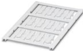
Conductor marker, Sheet, white, Unlabeled, Can be labeled with: BLUEMARK CLED, BLUEMARK LED, Plotter, Mounting type: Clip on, Cable diameter: 1.9-3.1 mm, Lettering field: 23 x 4 mm
