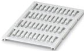
Conductor marker, Sheet, white, Unlabeled, Can be labeled with: BLUEMARK CLED, BLUEMARK LED, Plotter, Mounting type: Slide on, Cable diameter: 1.3-1.6 mm, Lettering field: 12 x 3 mm
