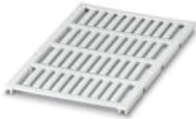
Conductor marker, Sheet, white, Unlabeled, Can be labeled with: BLUEMARK CLED, BLUEMARK LED, Plotter, Mounting type: Slide on, Cable diameter: 1.3-1.6 mm, Lettering field: 21 x 3 mm
