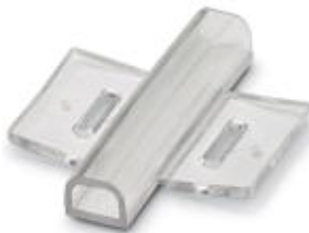
Cable marker carrier, transparent, Unlabeled, Horizontal, Mounting type: Insert, Cable diameter: >10 mm, Lettering field: 30 x 4 mm
