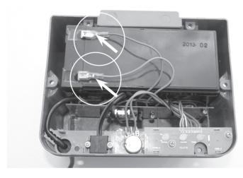
We recommend to exchange the accumulator approx. every 2 years. A new identical in construction accumulator is available from the manufacturer or dealer
