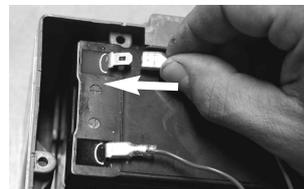
2. Place the electrical connector on the red (brown) cable onto the positive terminal of the rechargeable battery.
