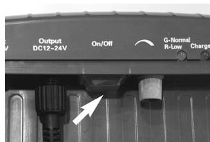
**2. Position 0 (OFF) :** The pump is switched-off. The accumulator is charged via the solar module and the electric energy is stored. The yellow LED is lit up as soon as the accumulator is charged via the solar module.
