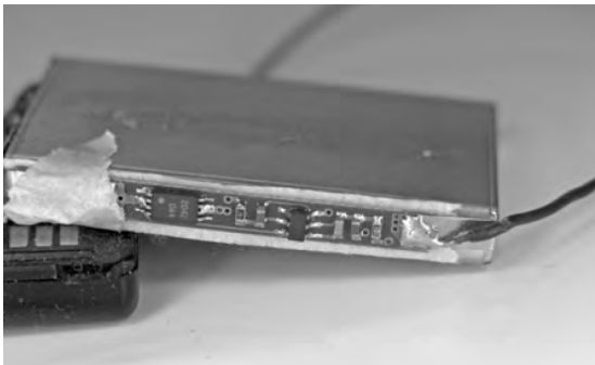
Fig. 038: Suitable rechargeable battery with integrated safety/protection electronics
