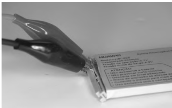
Fig. 039: Clamping connection with the rechargeable battery contacts
