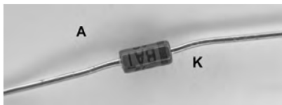
Fig. 005: a) Schottky diode, b) its circuit symbol
