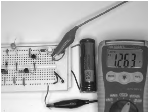
Fig. 034: Setup for measuring impulse charging with a multimeter
