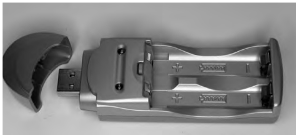
Fig. 023: Compact USB-charger for AA and AAA rechargeable batteries of types NiMH and NiCd
