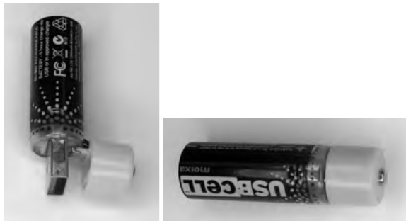
Fig. 022: USB-cell-NiMH, mignon cell with integrated USB adapter
