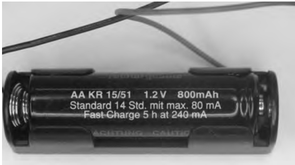
Fig. 028: Charging recommendation for one rechargeable battery: Constant current charge
