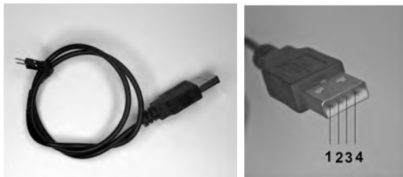
Fig. 002: USB connection cable, connection assignment of the plug: 1 = GND, 2 = D+, 3 = D-, 4 = +5 V
