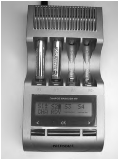
Fig. 035: Professional charger nickel-zinc, for AA and AAA cells
