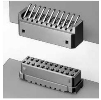
This 1.25mm (.049") pitch dual-in-line connector allows high-density packaging. Double-sided, high-pressure contacts and a housing locking feature provide reliable connections.
