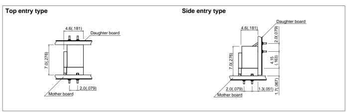
Note: The daughter board must be secured by means other than the connector. Contact JST for more details.
