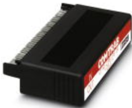
LSA-PLUS plug (COMTRAB CT 10) with surge voltage coarse and fine protection for 10 floating signal circuits. Nominal voltage: 24 V DC/AC version: 10 double wires
