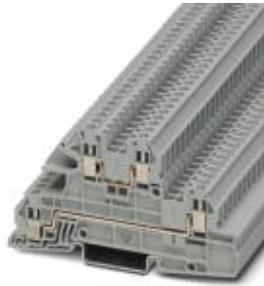
Installation level terminal block, Screw connection, Cross section: 0.2 mm 2 - 4 mm 2 , AWG: 24 - 12, Width: 5.2 mm, Color: gray, Mounting type: NS 35/7,5, NS 35/15
