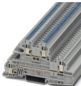
Installation level terminal block, Screw connection, Cross section: 0.2 mm 2 - 4 mm 2 , AWG: 24 - 12, Width: 5.2 mm, Color: gray, Mounting type: NS 35/7,5, NS 35/15
