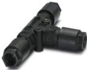
QUICKON T-distributor, black, 4+PE-pos., 1.0 mm 2 ... 2.5 mm 2 /690 V/20 A, for cable diameter of 6 mm ... 11 mm, with three QUICKON nuts
