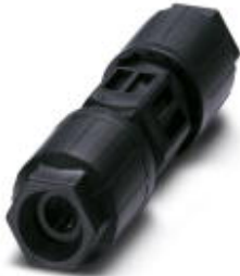
QUICKON cable connector, black, 4+PE-pos., 1.0 mm 2 ... 2.5 mm 2 / 690 V / 20 A, for 6 mm ... 11 mm cable diameter.
