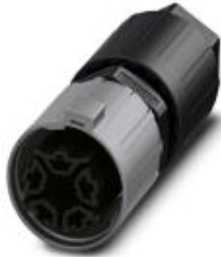
QUICKON connector, black, 4+PE-pos., 1.0 mm 2 ... 2.5 mm 2 /690 V/20 A, with QUICKON nut, for cables with 6 mm ... 11 mm diameter.
