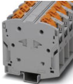
Feed-through terminal block, Connection method: Push-in connection, Cross section: 25 mm 2 - 95 mm 2 , AWG: 4 - 3/0, Width: 25 mm, Color: gray, Mounting type: NS 35/15
