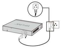
Figure 3-2 Connecting to the Ground
