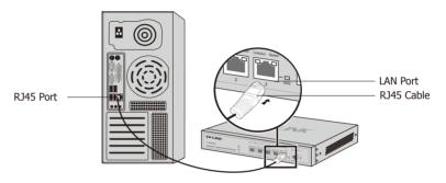
Figure 4-1 Connecting the LAN Port
