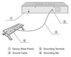
Figure 3-1 Connecting to the Grounding Bar
