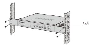
Figure 2-3 Rack Installation
