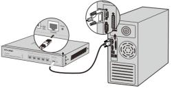
Figure 4-2 Connecting the Console Port
