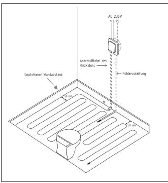
Thermostat controller and floor sensor:
