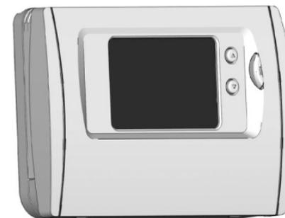
Place cover on thermostat and press until it snaps in place
