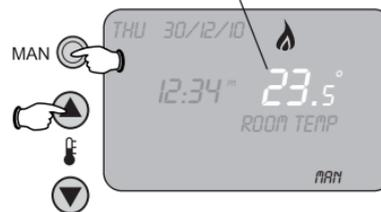
Press the mode buttons to select how the thermostat operates:
