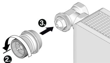
2. Turn the adjustment dial of the valve baseplate anti-clockwise until it stops.
