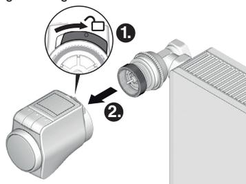
1. Unlock the radiator controller. To do so, slide the slide at the radiator controller towards the ☒.
