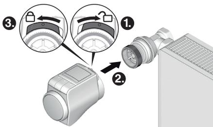
1. Ensure that the slide at the radiator controller is in the open position.
