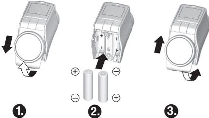
1. Move the front part slightly upwards and remove it downwards.
