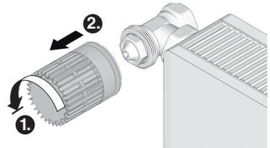
1. Turn the old thermostat head to the left until it stops and loosen the mounting.
