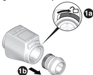
1. Separate the valve baseplate from the radiator controller. To do so, slide the slide towards the
