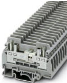
Test disconnect terminal block, Connection method: Screw connection, Cross section: 0.5 mm 2 -10 mm 2 , AWG: 20 - 10, Width: 8.2 mm, Mounting type: NS 35/7,5, NS 35/15, NS 32, Color: gray
