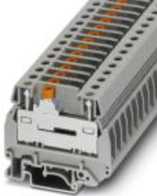
Slide-type terminal block, Connection method: Screw connection, Cross section: 0.5 mm 2 -10 mm 2 , AWG: 20 - 10, Width: 8.2 mm, Mounting type: NS 35/7,5, NS 35/15, NS 32, Color: gray
