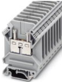
Feed-through terminal block, Connection method: Screw connection, Cross section: 0.5 mm 2 - 10 mm 2 , AWG: 20 - 8, Width: 10.2 mm, Color: gray, Mounting type: NS 35/7,5, NS 35/15, NS 32
