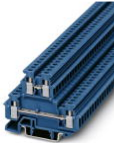
Feed-through terminal block, Cross section: 0.2 mm 2 - 4 mm 2 , AWG: 24 - 12, Connection type: Screw connection, Width: 5.2 mm, Color: blue, Mounting type: NS 15
