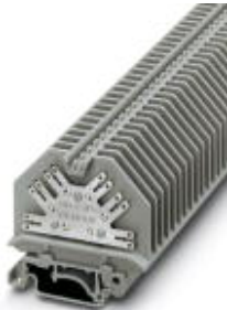
Feed-through terminal block, Connection method: Slip-on connection, Cross section: 0.5 mm 2 - 6 mm 2 , AWG: 20 - 10, Width: 6.2 mm, Color: gray, Mounting type: NS 35/7,5, NS 35/15, NS 32
