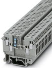
Feed-through terminal block, Connection method: Screw connection, Cross section: 0.2 mm 2 - 6 mm 2 , AWG: 24 - 10, Width: 6.2 mm, Color: gray, Mounting type: NS 35/7,5, NS 35/15, NS 32
