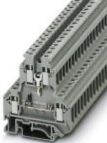
Component terminal block, Connection method: Screw connection, Cross section: 0.2 mm 2 - 4 mm 2 , AWG: 24 - 12, Width: 6.2 mm, Color: gray, Mounting type: NS 35/7,5, NS 35/15, NS 32
