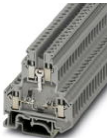
Component terminal block, Cross section: 0.2 mm 2 - 4 mm 2 , AWG: 24 - 12, Connection type: Screw connection, Width: 6.2 mm, Color: gray, Mounting type: NS 35/7,5, NS 35/15, NS 32
