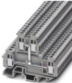
Feed-through terminal block, Cross section: 0.2 mm 2 - 4 mm 2 , AWG: 24 - 12, Connection type: Screw connection, Width: 5.2 mm, Color: gray, Mounting type: NS 15
