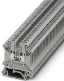
Feed-through terminal block, Connection method: Screw connection, Cross section: 0.2 mm 2 - 4 mm 2 , AWG: 24 - 12, Width: 5.2 mm, Color: gray, Mounting type: NS 32, NS 35/15, NS 35/7,5
