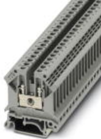
Feed-through terminal block, Connection method: Screw connection, Cross section: 0.2 mm 2 - 4 mm 2 , AWG: 24 - 10, Width: 6.2 mm, Color: gray, Mounting type: NS 35/7,5, NS 35/15, NS 32
