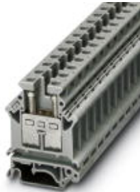
Feed-through terminal block, Connection method: Screw connection, Cross section: 0.5 mm 2 - 16 mm 2 , AWG: 20 - 6, Width: 10.2 mm, Color: gray, Mounting type: NS 35/7,5, NS 35/15, NS 32
