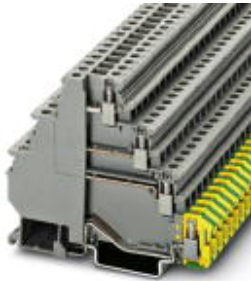
Feed-through terminal block, Cross section: 0.2 mm 2 - 4 mm 2 , AWG: 24 - 12, Connection type: Screw connection, Width: 6.2 mm, Color: gray, Mounting type: NS 35/7,5, NS 35/15
