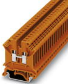
Feed-through terminal block, Connection method: Screw connection, Cross section: 0.2 mm 2 - 6 mm 2 , AWG: 24 - 10, Width: 6.2 mm, Color: orange, Mounting type: NS 35/7,5, NS 35/15, NS 32
