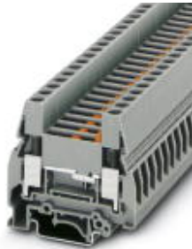
Disconnect terminal block, Connection method: Screw connection, Cross section: 0.5 mm 2 -16 mm 2 , AWG: 20 - 8, Width: 8.2 mm, Mounting type: NS 35/7,5, NS 35/15, NS 32, Color: gray
