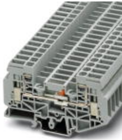
Test disconnect terminal block, Connection method: Screw connection, Cross section: 0.5 mm 2 -10 mm 2 , AWG: 20 - 10, Width: 8.2 mm, Mounting type: NS 35/7,5, NS 35/15, NS 32, Color: gray
