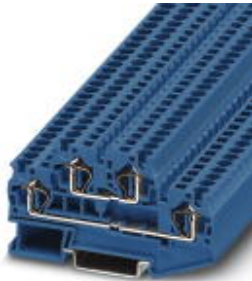
Feed-through terminal block, Cross section: 0.08 mm 2 - 6 mm 2 , AWG: 28 - 10, Connection type: Spring-cage connection, Width: 6.2 mm, Color: blue, Mounting type: NS 35/7,5, NS 35/15
