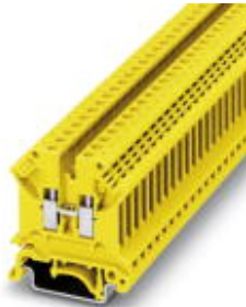
Feed-through terminal block, Connection method: Screw connection, Cross section: 0.2 mm 2 - 6 mm 2 , AWG: 24 - 10, Width: 6.2 mm, Color: yellow, Mounting type: NS 35/7,5, NS 35/15, NS 32
