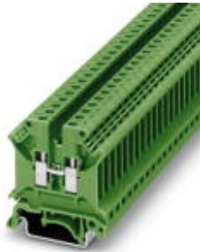
Feed-through terminal block, Connection method: Screw connection, Cross section: 0.2 mm 2 - 6 mm 2 , AWG: 24 - 10, Width: 6.2 mm, Color: green, Mounting type: NS 35/7,5, NS 35/15, NS 32
