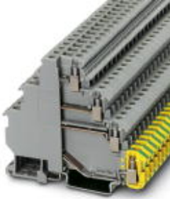
Sensor/actuator terminal block, Cross section: 0.2 mm 2 - 4 mm 2 , AWG: 24 - 12, Connection type: Screw connection, Width: 6.2 mm, Color: gray, Mounting type: NS 35/7,5, NS 35/15
