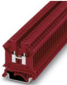
Feed-through terminal block, Connection method: Screw connection, Cross section: 0.2 mm 2 - 6 mm 2 , AWG: 24 - 10, Width: 6.2 mm, Color: red, Mounting type: NS 35/7,5, NS 35/15, NS 32
