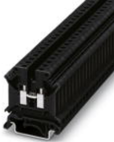
Feed-through terminal block, Connection method: Screw connection, Cross section: 0.2 mm 2 - 6 mm 2 , AWG: 24 - 10, Width: 6.2 mm, Color: black, Mounting type: NS 35/7,5, NS 35/15, NS 32
