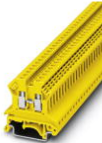
Feed-through terminal block, Connection method: Screw connection, Cross section: 0.2 mm 2 - 4 mm 2 , AWG: 24 - 14, Width: 5.2 mm, Color: yellow, Mounting type: NS 35/7,5, NS 35/15
