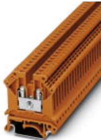
Feed-through terminal block, Connection method: Screw connection, Cross section: 0.2 mm 2 - 4 mm 2 , AWG: 24 - 12, Width: 5.2 mm, Color: orange, Mounting type: NS 32, NS 35/15, NS 35/7,5
