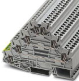
Feed-through terminal block, Connection method: Spring-cage connection, Cross section: 0.08 mm 2 - 4 mm 2 , AWG: 28 - 12, Width: 5.2 mm, Color: gray, Mounting type: NS 35/7,5, NS 35/15
