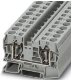
Feed-through terminal block, Connection method: Spring-cage connection, Cross section: 0.2 mm 2 - 25 mm 2 , AWG: 24 - 4, Width: 12.2 mm, Color: gray, Mounting type: NS 35/15, NS 35/7,5
